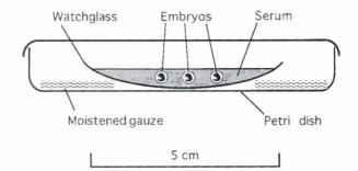
Fig. 1. Watchglass culture apparatus: several of these can be stacked in a gas-tight chamber within the incubator.
