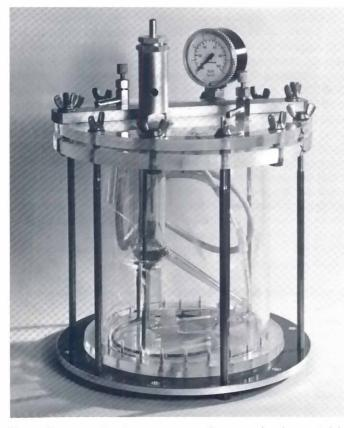
Fig. 4. Pressure chamber apparatus. Pressure chamber containing circulators that can operate at two or three atmospheres of pressure.
