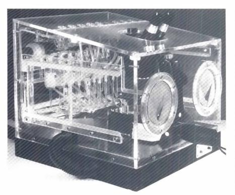
Fig. 3. Incubator for circulator cultures. Purpose made incubator housing circulators and a binocular microscope.
