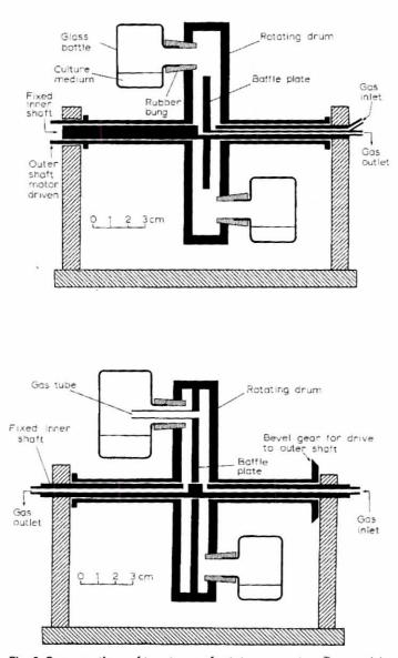
Fig. 6. Cross sections of two types of rotator apparatus. Two models of rotator apparatus, in which the rotating bottles are constantly gassed by diffusion (upper diagram) or via tubes projecting into the bottles (lower diagram). (From New and Cockroft, 1979).
