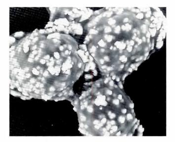
Fig. 6. Mineral induction by dentin phosphoprotein (DPP) at physiological ion concentrations *in vitro*. *DPP* was immobilized on agarose beads (8 mg ligand/g dry beads) and incubated for 24 h at a [Ca]x[P] product of 1.4 mM<sup>2</sup>. A strong induction of crystals can be seen (back-scattered electron imaging) both on and within the beads. The mineral can be identified as HAP by x-ray diffraction (Luusi et al., 1988).
