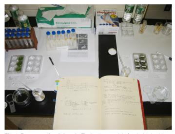
**Fig. 6. From a student's bench.** The basic materials for the Hydra bioassay used by a high school student to assess lead remediation by Lemna sp. The animals can be observed with magnifying glasses as shown here but also with a stereomicroscope, which is useful to precisely define the observed phenotypes.
