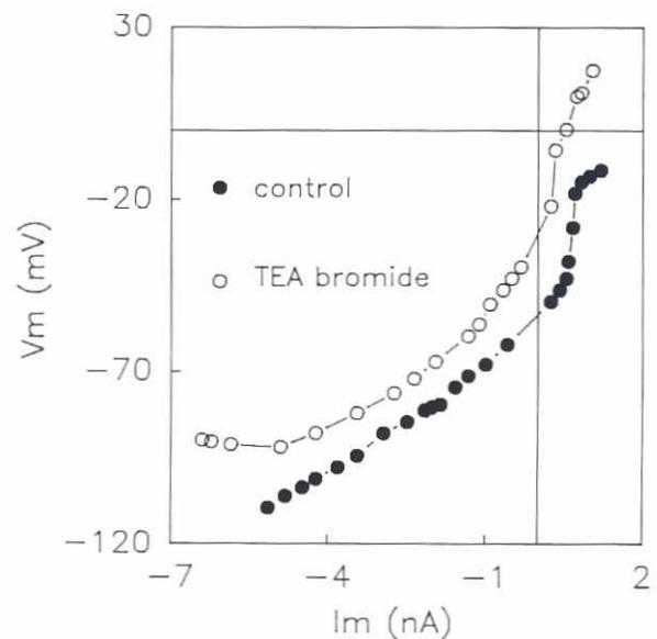
Fig. 13. Effect of 50 mM TEA bromide on the I/V curve recorded in current clamp.
