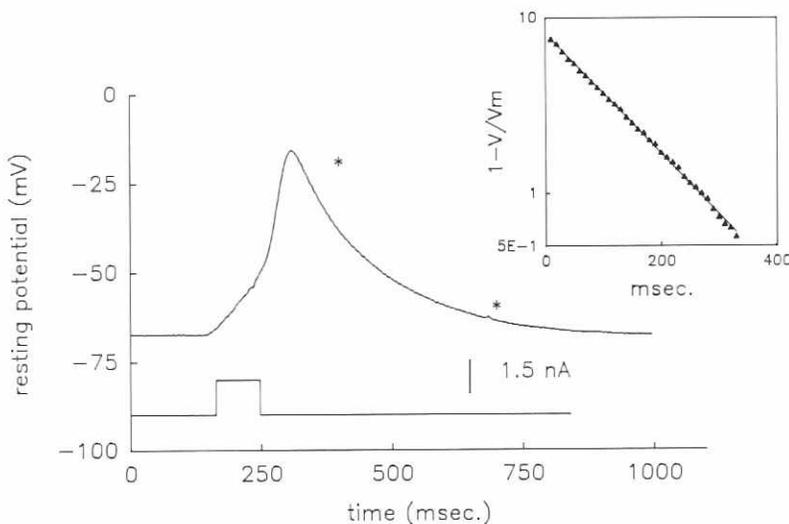
**Fig. 3. Action potential of an immature *Patella* oocyte obtained with a threshold depolarizing current.** The inset represents the semi-log plot of  $1-V/V_m$  vs time of the repolarizing phase of the action potential corresponding to the portion of curve between (\*).
