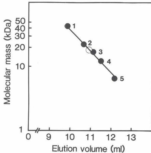
**Fig. 4.** Determination of molecular mass of intact p10. Purified p10 (6.6  $\mu$ g) was subjected to HPLC on a molecular sieve column of G3000SWxl with various marker proteins. Molecular mass is plotted against the elution volume. The following proteins were used for calibration of the column: 1, ovalbumin (45 kDa); 2, soybean trypsin inhibitor (22 kDa); 3, myoglobin (17 kDa); 4, cytochrome c (12.4 kDa); 5, aprotinin (6.5 kDa). The elution volume of p10 is shown by an open circle.
