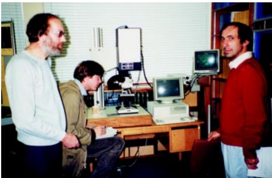
**Fig. 3. The *C. elegans* project spawned several technical developments such as a confocal microscope, which was developed to study the cytoarchitecture of the developing *C. elegans* embryo. This is the commercial prototype a few hours after it was first made to work after an all night effort. John White (right), Richard Durbin (centre) and Mick Fordham (left).**
